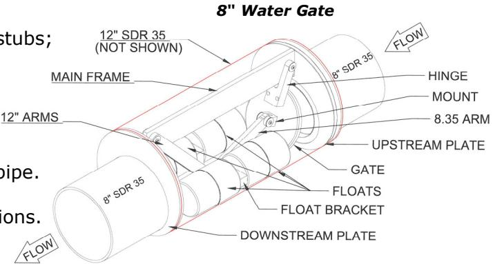
\*To minimize seepage, we recommend installing 20' of non-perforated pipe on the upstream side of the Water Gate, or using an Anti-Seep Collar below the Water Gate.
