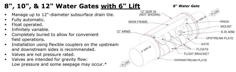
\*To minimize seepage, we recommend installing 20' of non-perforated pipe on the upstream side of the Water Gate, or using an Anti-Seep Collar below the Water Gate.
